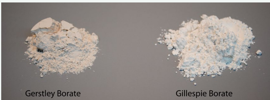
Raw Samples of Gerstley borate and Gillespie borate. Gerstley borate is a light tan/off white, whereas Gillespie borate is bright white.
